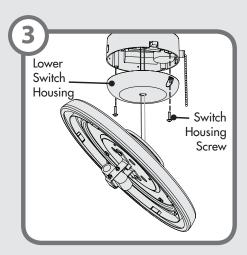
Lift the lower switch housing up so that the screw holes line up with the holes in the upper switch housing. Install the switch housing screws and tighten securely.
